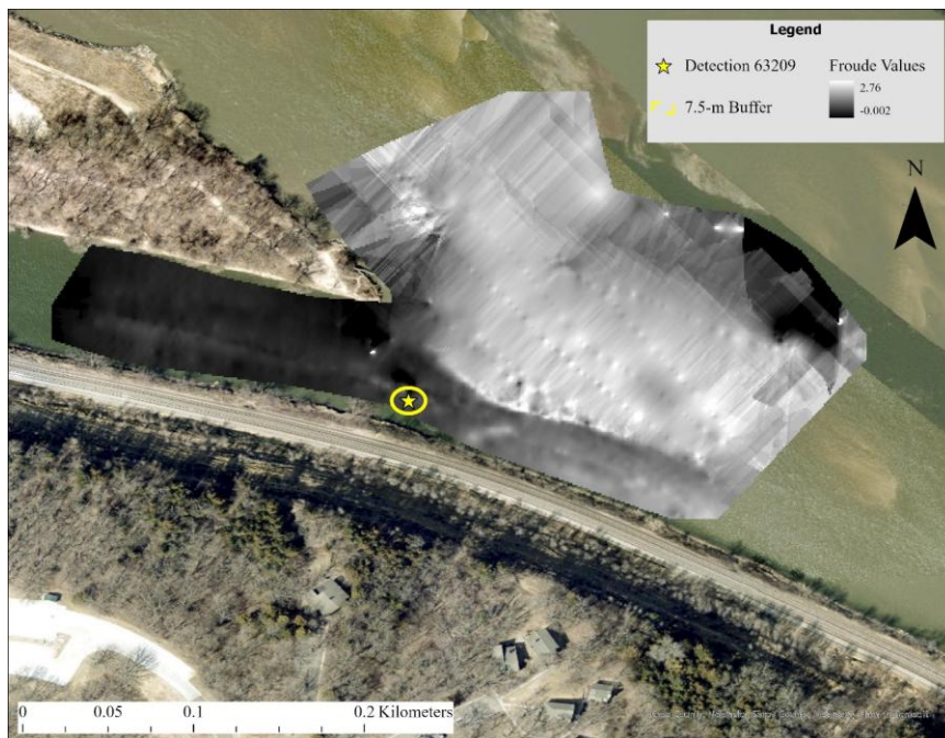
Figure 12. An example of a Froude value map derived from the depth and velocity raster maps (Figure 11) generated in ArcGIS Pro.
