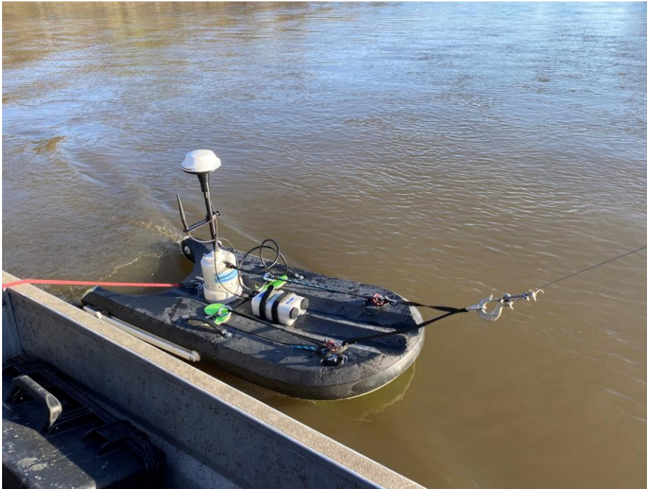
Figure 10. The ADCP mounted to side of the airboat. Transducer is approximately 3 cm below the rig to measure depth and velocity.
